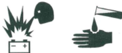
The battery contains acidic substances, so you should wear protective clothing and glasses when using the battery.
