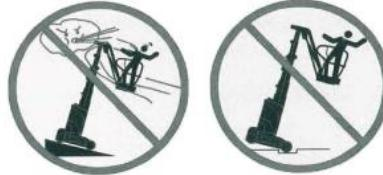
Do not use the platform controller to release the platform when the platform is stuck or other nearby objects hinder its normal movement. All personnel must leave the platform before attempting to release the platform using ground control.
